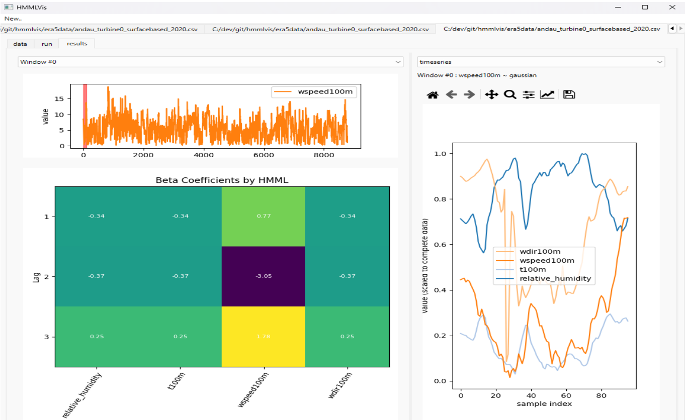
Figure 3. Application Showcase 3/7: Initial results view for window index 0. Top-Left: Time-series of the target variable for the window selected in the dropdown window. Bottom-Left: heatmap of beta coefficients. The values in the grid represent the beta-coefficients introduced in section 2. The colors are applied by a mapping of these coefficients using matplotlib’s viridis colormap, indicating in this case (1) a low influence of the dark green variables, (2) a strong negative influence of wind-speed at a lag of 2 by dark purple, and (3) a strong positive influence of wind-speed at lag 1. Right: scaled time-series data for the selected window. Unlike the heatmap, the colors for this plot are selected randomly to visually distinguish the variables.
