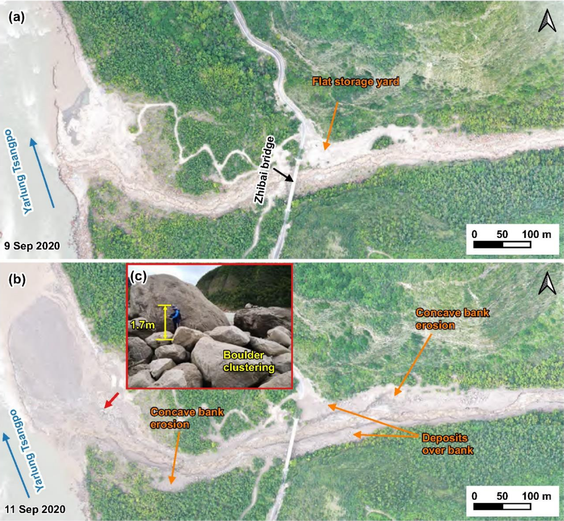
Figure 7: Comparison of pre-and post-event aerial photos on the downstream channel and alluvial fan. (a) the UAV photo on 9 September 2020; (b) the UAV photo on 11 September 2020; (c) On-site picture of the boulder clustering on 11 September 2020 (the camera angle direction is denoted by red arrow in figure b).
