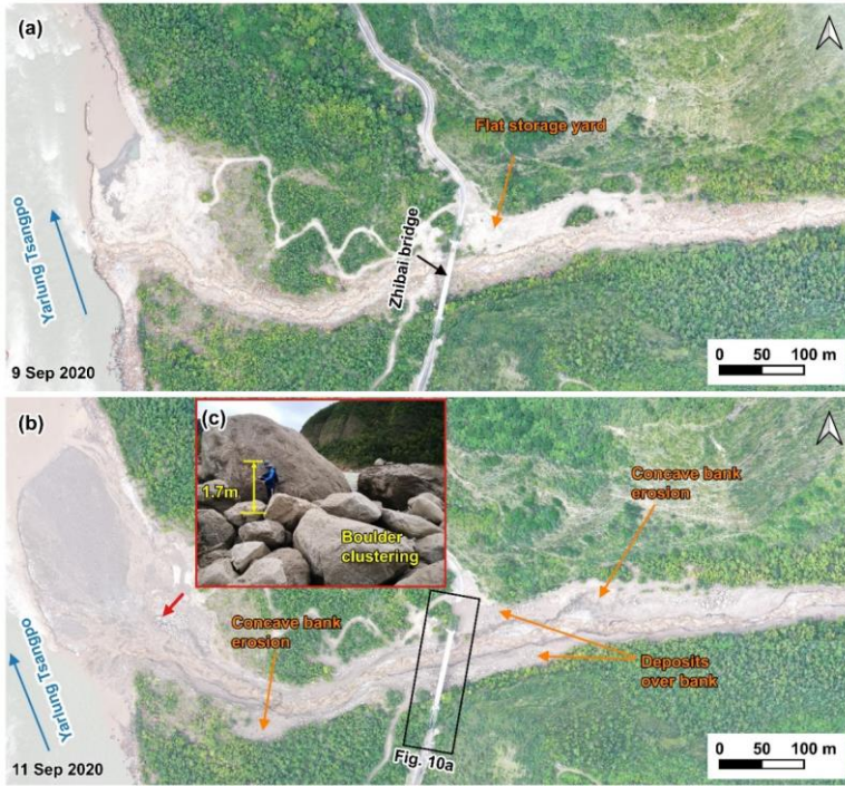
Figure 7: Comparison of pre-and post-event aerial photos on the downstream channel and alluvial fan. (a) the UAV photo on 9 September 2020; (b) the UAV photo on 11 September 2020; (c) On-site picture of the boulder clustering on 11 September 2020 (the camera angle direction is denoted by red arrow in figure b).
