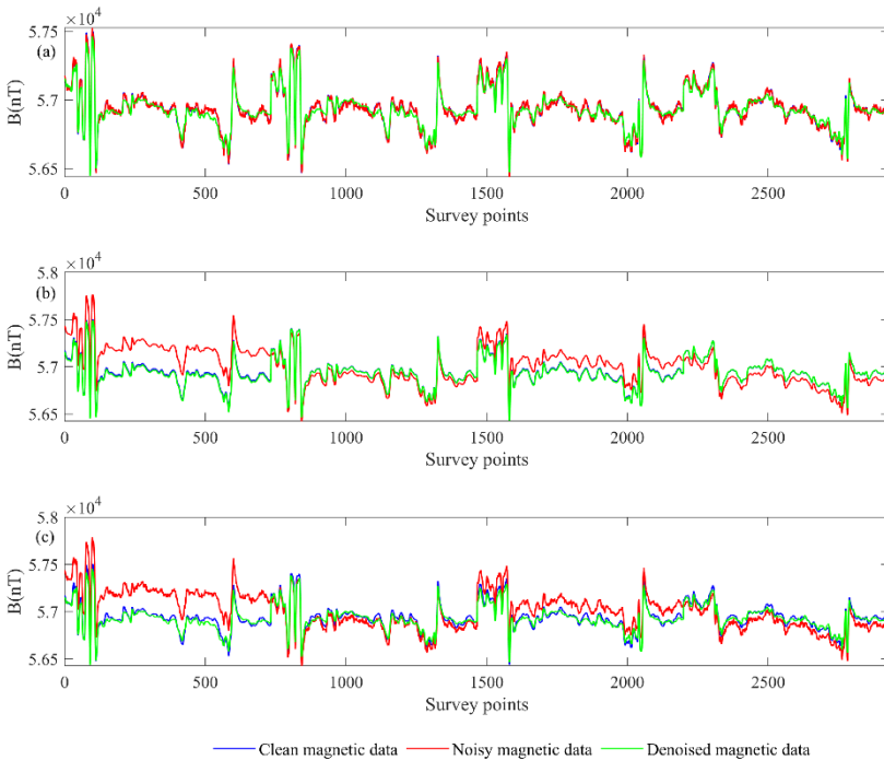
205 Figure 3: Leveling result analysis of synthetic airborne magnetic data. (a) Magnetic data with Gaussian white noises. (b) Magnetic data with leveling errors. (c) Magnetic data with Gaussian white noises and leveling errors.
