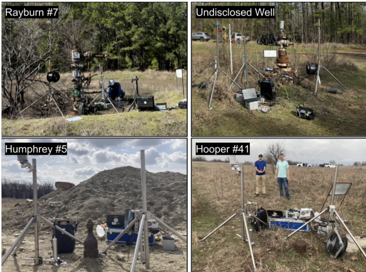
Figure 6: Wells measured in Lufkin, Texas (top) and Barnsdall, Oklahoma (bottom) using the FAST method. Both wells in Texas were of the “christmas tree” variety (multiple potential leak points) and were measured using No Fan and Low Fan speeds because the background wind speeds were < 1 m/s. Both wells in Oklahoma were lower to the ground, had only one leak point and were measured with No Fan, Low Fan and High Fan speeds due to the higher background winds ( > 1 m/s).
