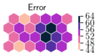
Figure 5: RMSE error, i.e. mean distance between instantaneous snapshots and the weight matrix of its best matching cluster, averaged by cluster. This is now a panel on the main text's figure 6.
