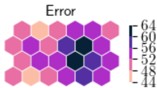
Figure 5: RMSE error, i.e. mean distance between instantaneous snapshots and the weight matrix of its best matching cluster, averaged by cluster. This is now a panel on the main text's figure 6.
