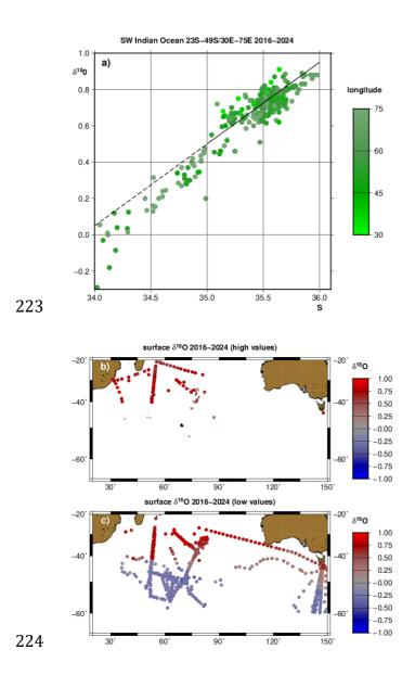
Figure 3: (a) S- $\delta^{18}$ O scatter diagram of 0-30m LOCEAN data within the southwestern region (30-75°E/23-49°S) coloured as a function of longitude, with the regression line (black line) of the data in S- $\delta^{18}$ O space for the 35-36 range in practical salinity. The spatial distributions of the LOCEAN data with higher and lower  $\delta^{18}$ O relative to that regression line in the whole Indian Ocean north of 60°S are shown on panels (b) and (c), respectively.
