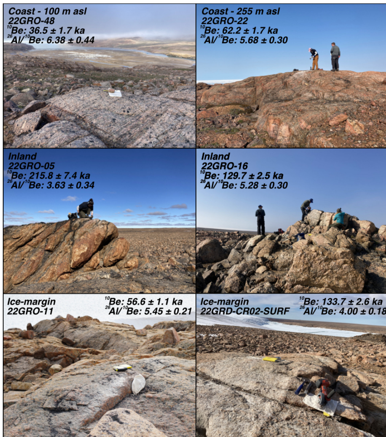
Figure 8: subset of bedrock sample photos and resultant cosmogenic nuclide results. Note the smoothness of the coastal outcrops compared to the rough, weathered textures of the inland and ice-margin sites.
