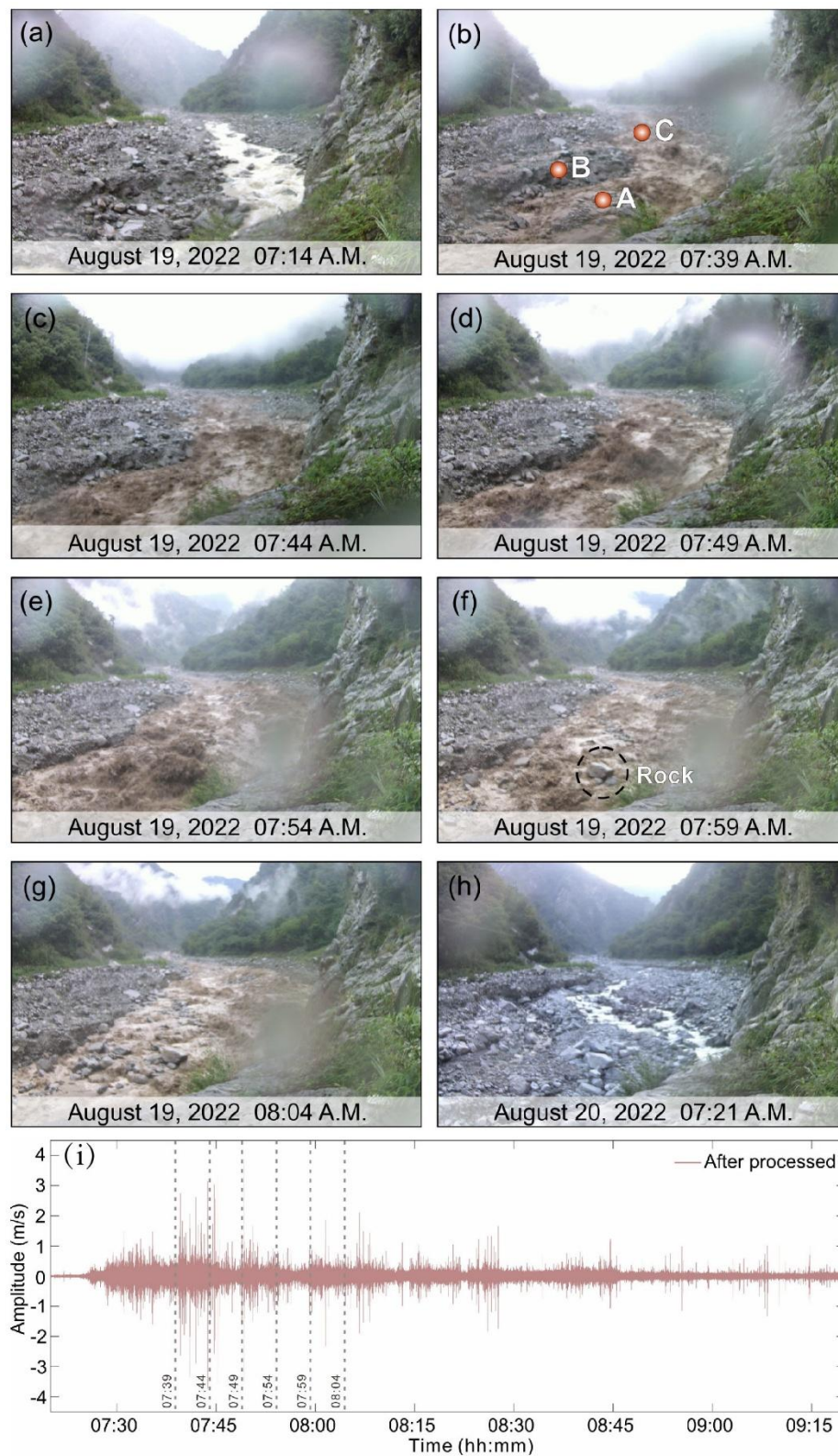
Fig. 7. Infrared camera images taken and the seismic signal recorded at monitoring station 1 in Fotangba Gully during the second debris flow on the morning of August 19, 2022. Images were recorded every 5 minutes: (a) 7:14 frame (b) 7:39 frame; (c) 7:44 frame; (d) 7:49 frame; (e) 7:54 frame; (f) 7:59 frame; (g) 8:04 frame; (h) August 20, 2022, 8:04 Frame; (i) seismic signal recorded at the point.
