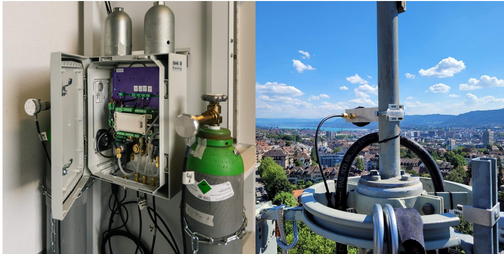
Figure A1. Examples of the \text{CO}_2 sensor's typical installations in the CARIN-ZH sensor network in Zürich city. The photograph on the left was taken by Pekka Pelkonen from ICOS RI.
