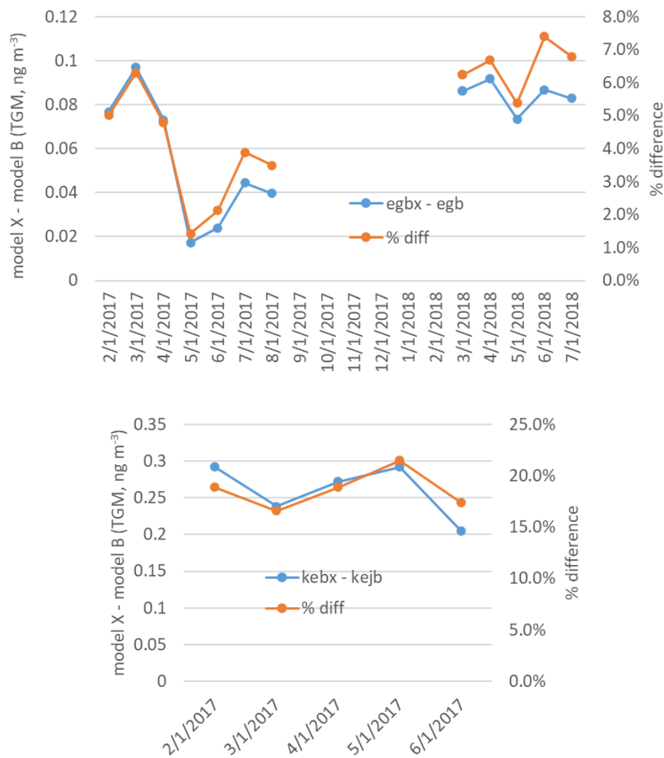
Figure S13S11: Intercomparison between Tekran model X and B measurements for EGB (top) and KEJ/KEB (bottom). Absolute and relative differences for hourly measurements are plotted.
