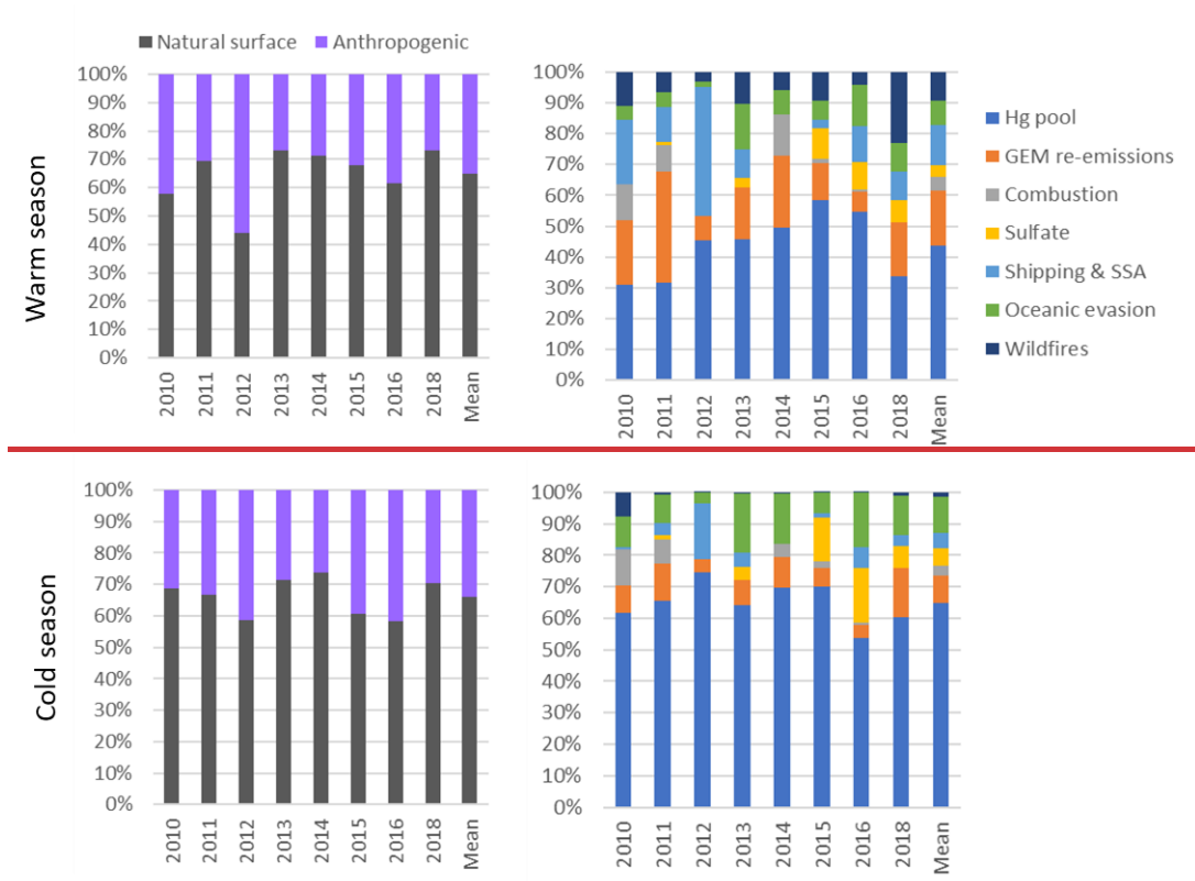
Figure S2: Relative source contributions to warm and cold season mean TGM at SAT. Mean applies to the 2010-2018 period except 2017. Warm season: May to Oct; cold season: Nov to Apr. Natural surface emissions comprise wildfires, GEM re-emissions, oceanic evasion, and natural surface emissions contributing to the Hg pool. Anthropogenic emissions comprise local combustion; sulfate, and anthropogenic emissions contributing to the Hg pool.
