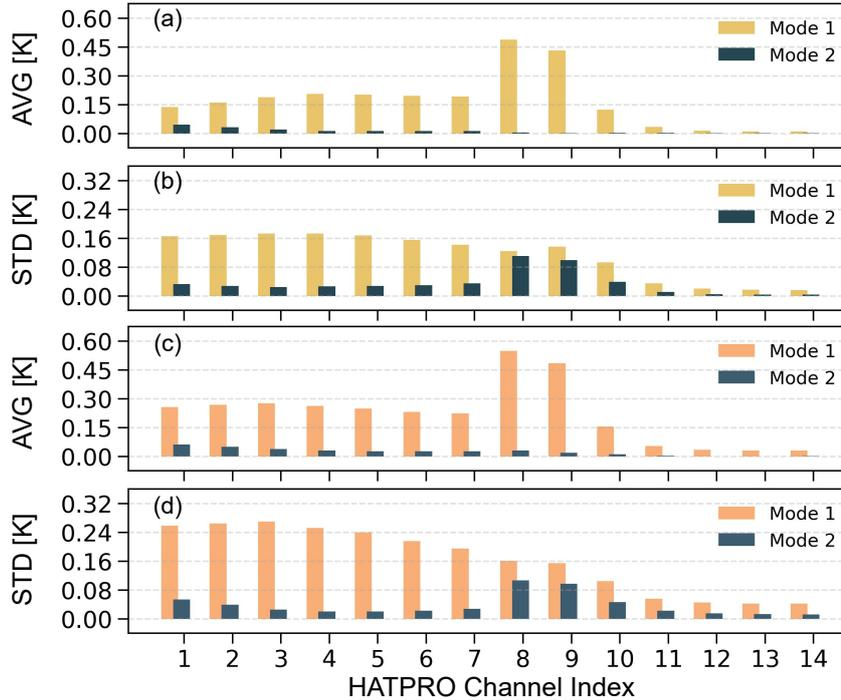
**Figure 2.** (a) and (b): AVGs and STDs of simulated BTs at 7 observed zenith angles in HATPRO channels. RT simulations for both interpolation mode 1 and 2 performed under the 54L ECMWF [83-83-profile](#) dataset. MonoRTM serves as a benchmark to provide reference values for comparison. (c) and (d): Same as (a) and (b), but with RT simulations performed under the 54L UMBC [48-48-profile](#) dataset.
