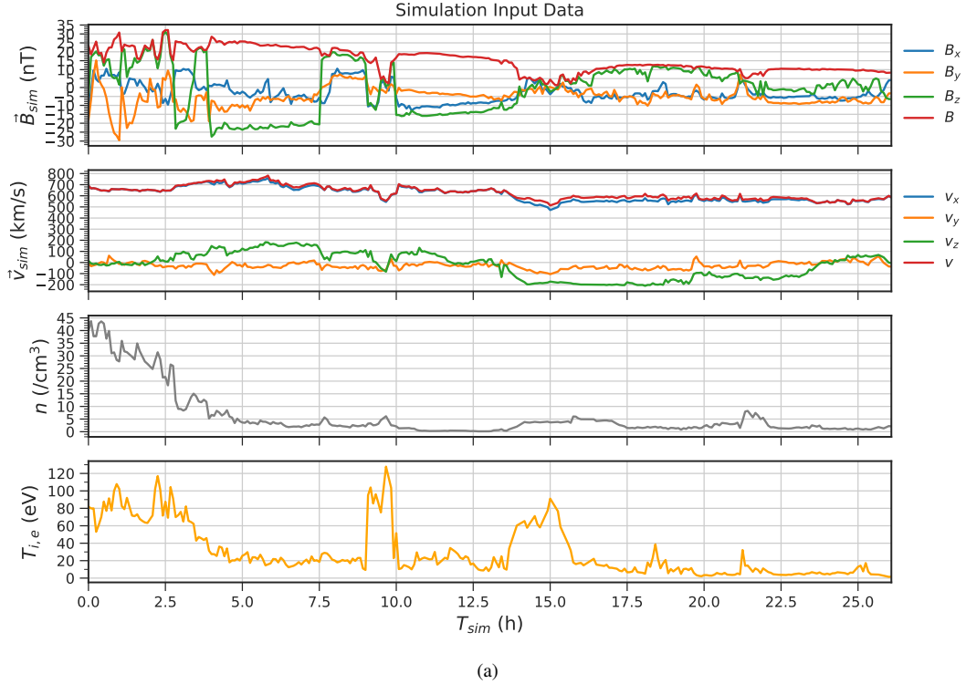
Figure 3. Upstream solar wind boundary conditions for the magnetospheric simulation. Time series of the solar wind parameters used as the initial and driving input for the Gorgon-Space MHD simulation, derived from the EUHFORIA heliospheric model. The data corresponds to the conditions at the Earth-Sun L1 point for the period beginning at 00:03 UT on June 23, 2015, coinciding with the arrival of the first CME. From top to bottom, the panels show: the three vector components of the magnetic field B (in nT) and plasma velocity V (in km/s), the plasma density (in \text{cm}^{-3} ), and the plasma temperature T (in eV). All vector components are presented in the Geocentric Solar Ecliptic (GSE) coordinate system.
