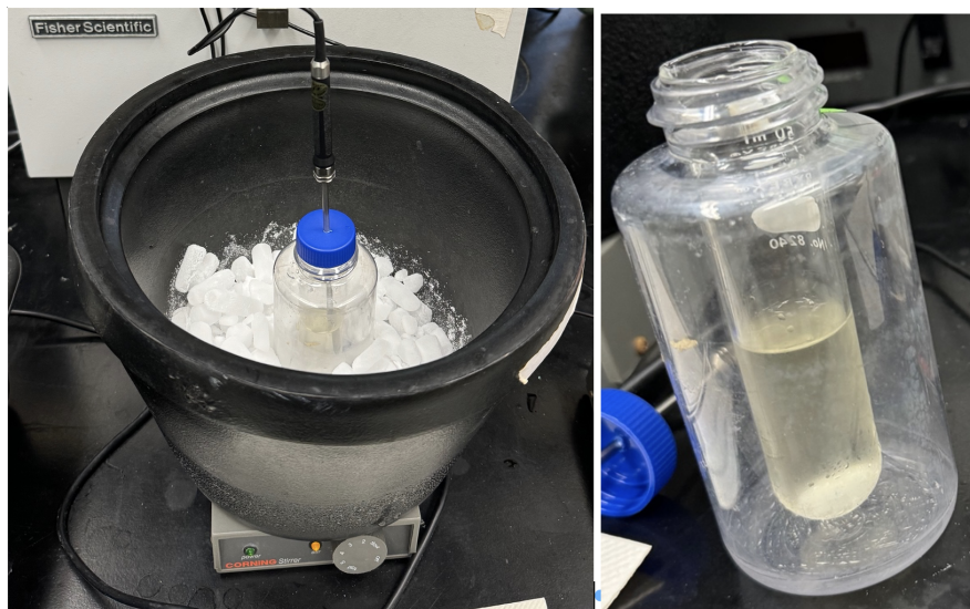
Figure 1. Freezing point measurement apparatus. (Left) the thermal calorimetric apparatus constituted of an isolated bucket on a magnetic stir plate. The bucket contains dry ice in which a chamber is placed. (Right) the chamber is composed of a 50 mL glass culture tube inside a polycarbonate 150 mL bottle.
