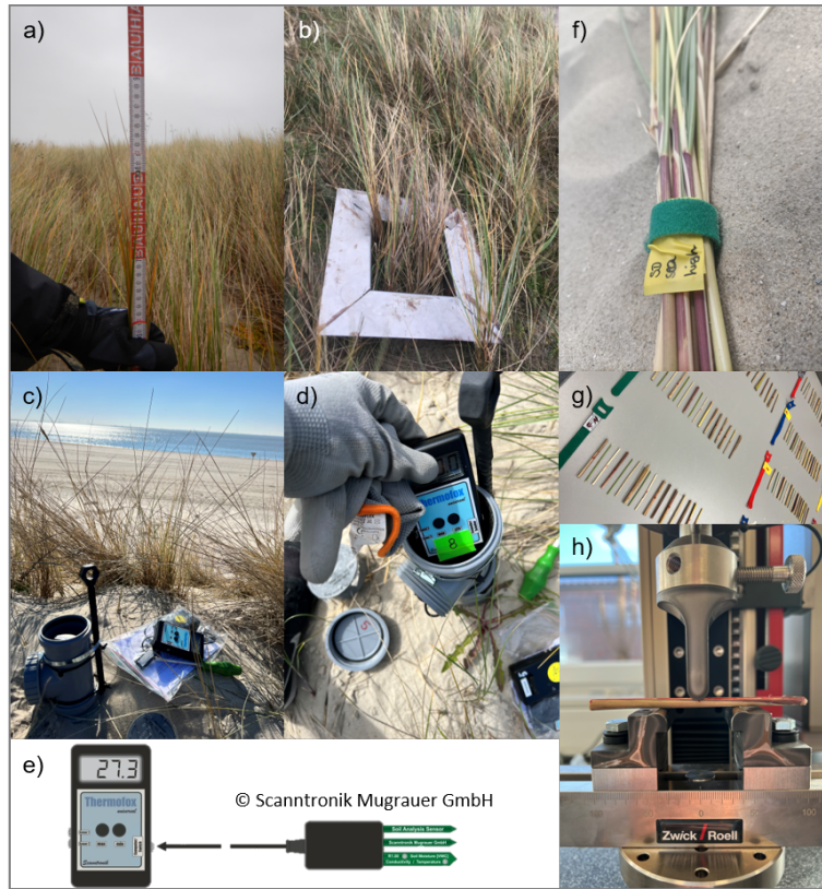
Figure A1. Overview of the methodology used in this study. (a) Measurement of canopy height using a folding ruler. (b) Determination of horizontal density with a 20 cm frame. (c) Replacement of the data logger connected to the soil analysis sensor, with a close-up view in (d) showing the data logger within its enclosure during replacement. (e) Manufacturer's overview (Scanntronik Mugrauer GmbH, 2024a) of the data logger (left) connected to the soil analysis sensor (right), which is installed approximately 20 – 30 cm deep in the soil. (f) Bundle of plant samples collected for further laboratory analysis. (g) Sample sections prepared for three-point bending tests. (h) Image of a sample in place for a three-point bending test before the start of the experiment.
