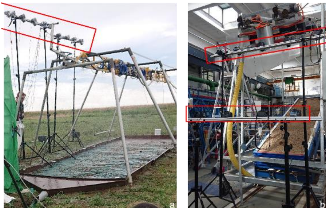
Figure 1: Rainfall simulator used in the field (a) and in the laboratory (b).
