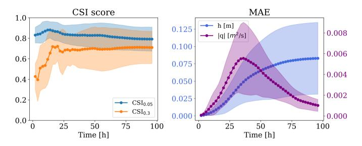
Figure 8. Temporal evolution of CSI scores (left) and MAE of water depth h and unit discharge q (right) for the test dataset. The confidence bands refer to 1 standard deviation from the mean.
