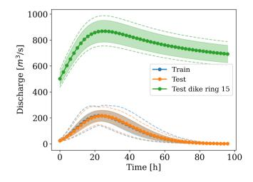
**Figure 6.** Distribution and shape of the hydrographs used as inputs for the training (blue), synthetic test (orange), and dike ring 15 test (green) simulations. The shaded region indicates one standard deviation away from the mean, at each time step. The dotted lines represent the envelopes of the minimum and maximum discharges at each time step.
