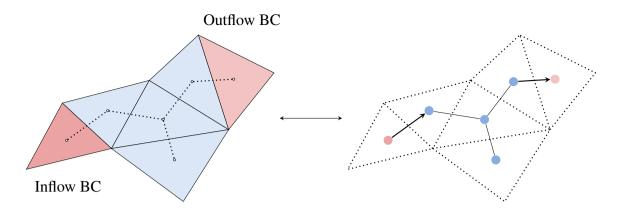
**Figure 3.** Schematic representation of an arbitrary triangular volume mesh (left) with a two ghost cell cells for inflow and outflow boundary conditions (leftBC). The ghost cell cells (red) is are added in correspondence of a boundary cell which receives a given boundary condition. In the dual graph (right), a directed edge is added from the ghost cell to the domain cell, or vice-versa, depending on whether the type of boundary condition is an inflow or an outflow, respectively.
