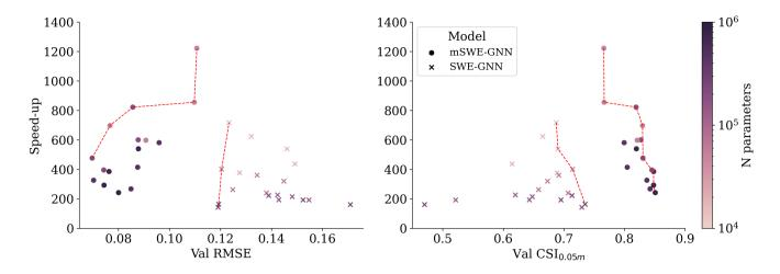
Figure 7. Pareto front of the mSWE-GNN and SWE-GNN models for speed-ups, validation RMSE (left), and validation CSI with 0.05 m water depth threshold (right). The models' size varies with number of hidden features and number of GNN layers.
