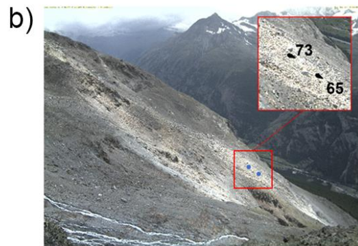
Figure 6: Validation principle illustrated through direct comparison of two measured point trajectories (ground truth) and their corresponding trajectories derived from time-lapse images. Illustration of the tracking principle used for 3D trajectory validation.
