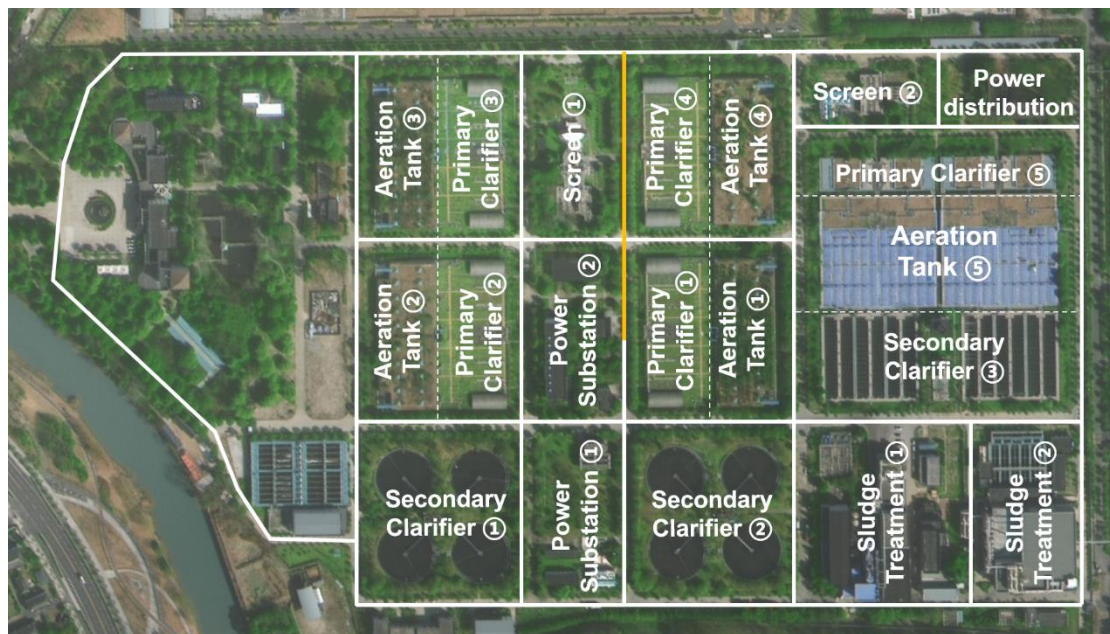
Figure 1. Distribution of functional areas of the WWTP. The yellow mark represents the simulated location of the line source. Solid lines show the roads measured by the mobile vehicle. Map data are from ESRI.
