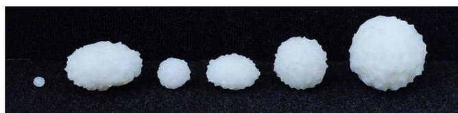
**Figure 5.** Six examples of 3D-printed hailstones in different sizes and forms.
