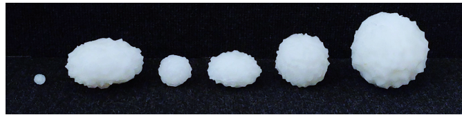
Figure 4. Six examples of 3D printed hailstones in different sizes and forms.
