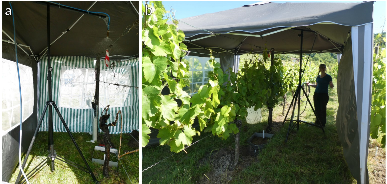
Figure 2: Installation of the portable Tübingen rainfall simulator in the vineyard with the runoff plots directly within the vine rows. (a) Tübingen rainfall simulator during rainfall simulation experiment in April in the vineyard without foliage. (b) Tübingen rainfall simulator during rainfall simulation experiment in June in the vineyard with foliage.
