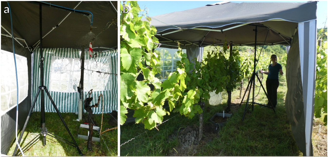
200 Figure 2: Installation of the portable Tübingen rainfall simulator in the vineyard with the runoff plots directly within the vine rows. (a) Tübingen rainfall simulator during rainfall simulation experiment in April in the vineyard without foliage. (b) Tübingen rainfall simulator during rainfall simulation experiment in June in the vineyard with foliage.
