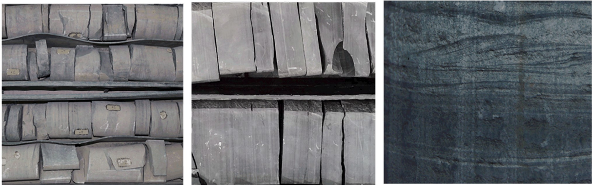
Figure 6 The tight sand containing thin shale beds. The light-colored sections of the core is tight sand, while the dark-striped sections are thin shale beds.
