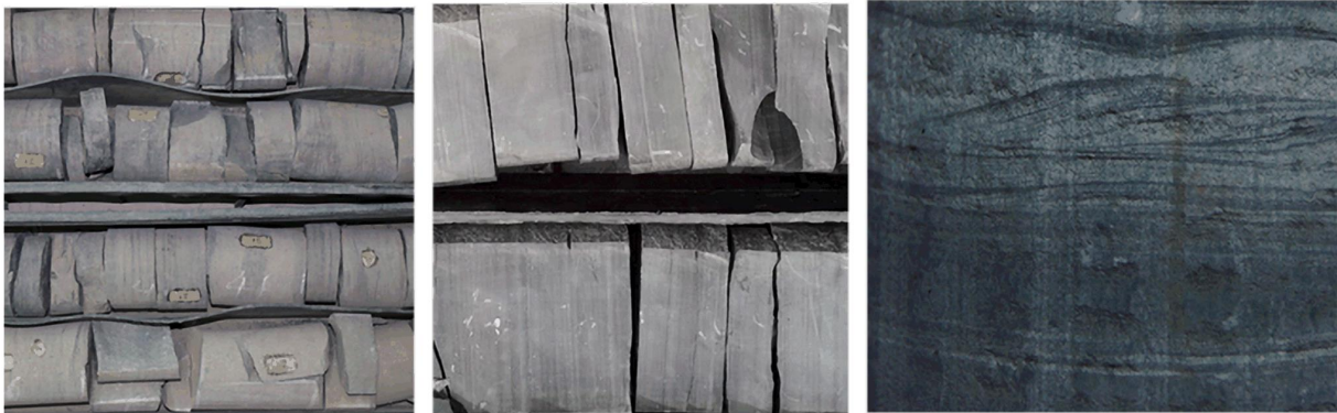
Figure 62 The tight sand containing thin shale beds. The light-colored sections of the core is tight sand, while the dark-striped sections are thin shale beds.
