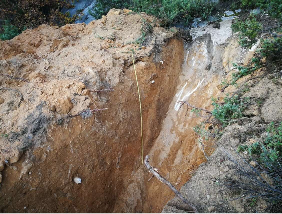
Figure S1. Northern wall of trench TA. Detail of the bedrock fault plane.
