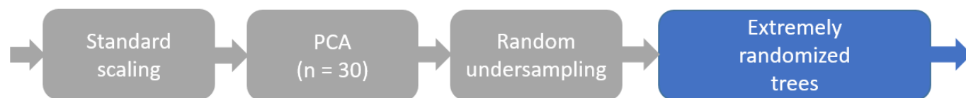
Figure 3. Block diagram describing the processing pipeline (the grey boxes) used in the ML model employed in this study, and the ML model chosen by TPOT (the blue box). This figure is an in-depth view of the 'Failure Prediction Model' shown in Fig. 2.
