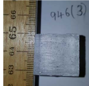
Figure S4: Picture of sample from RECAP bag 946 (2.2 x 2.2 x 2.4 cm) used to determine the average bubble diameter.
