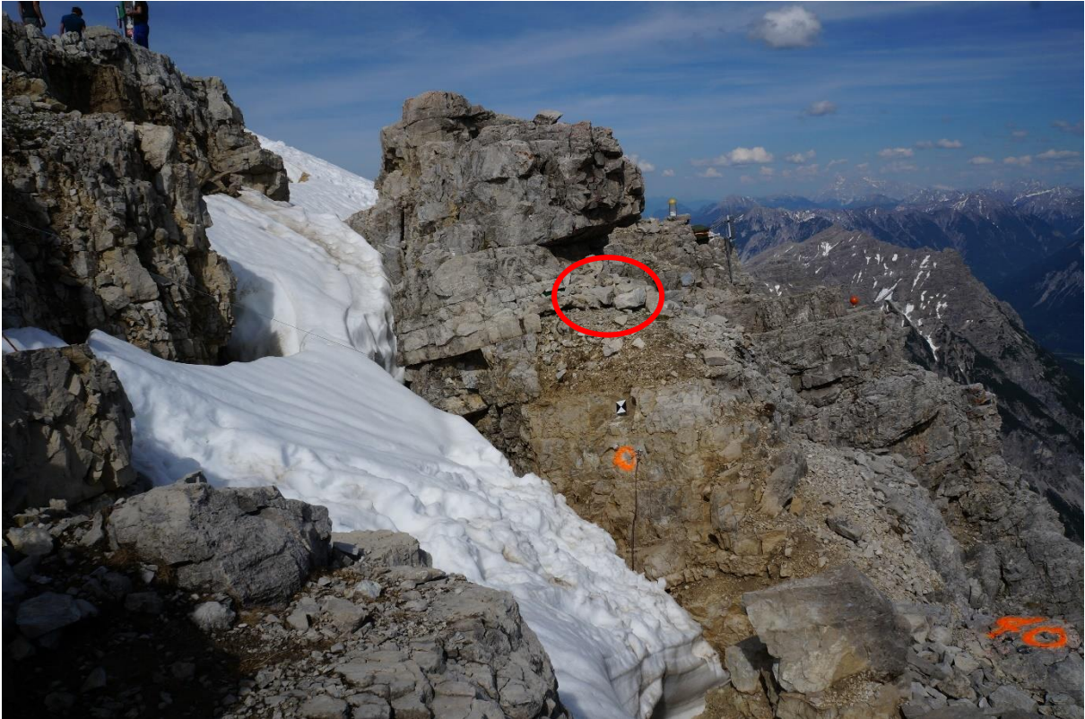
10 Fig. S 4: Photo of the main crack with position of seismic station HV 1 (red ellipse).
