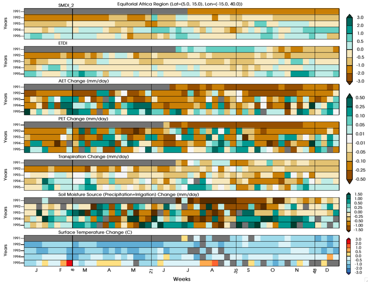
Figure 7. Spatially averaged drought indices (SMDI_2 & ETDI) and anomalies for other drivers (Actual and Potential Evapotranspiration, Transpiration, Moisture Source (Precipitation plus irrigation) and Surface Temperature) at weekly scale for the equatorial Africa region (Latitude = 5°-15° N, Longitude = 15° W- 40° E).
