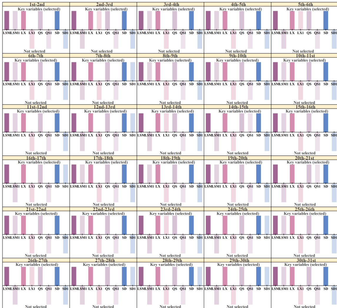
556 Figure 13. Key factors in the five-dimensional vine copula structure constructed in two adjacent days 557 (LSM, LX, QS, SD represent the runoff sequences of current day, while LSM1, LX1, QS1, SD1 represent the 558 runoff sequences of previous day)
