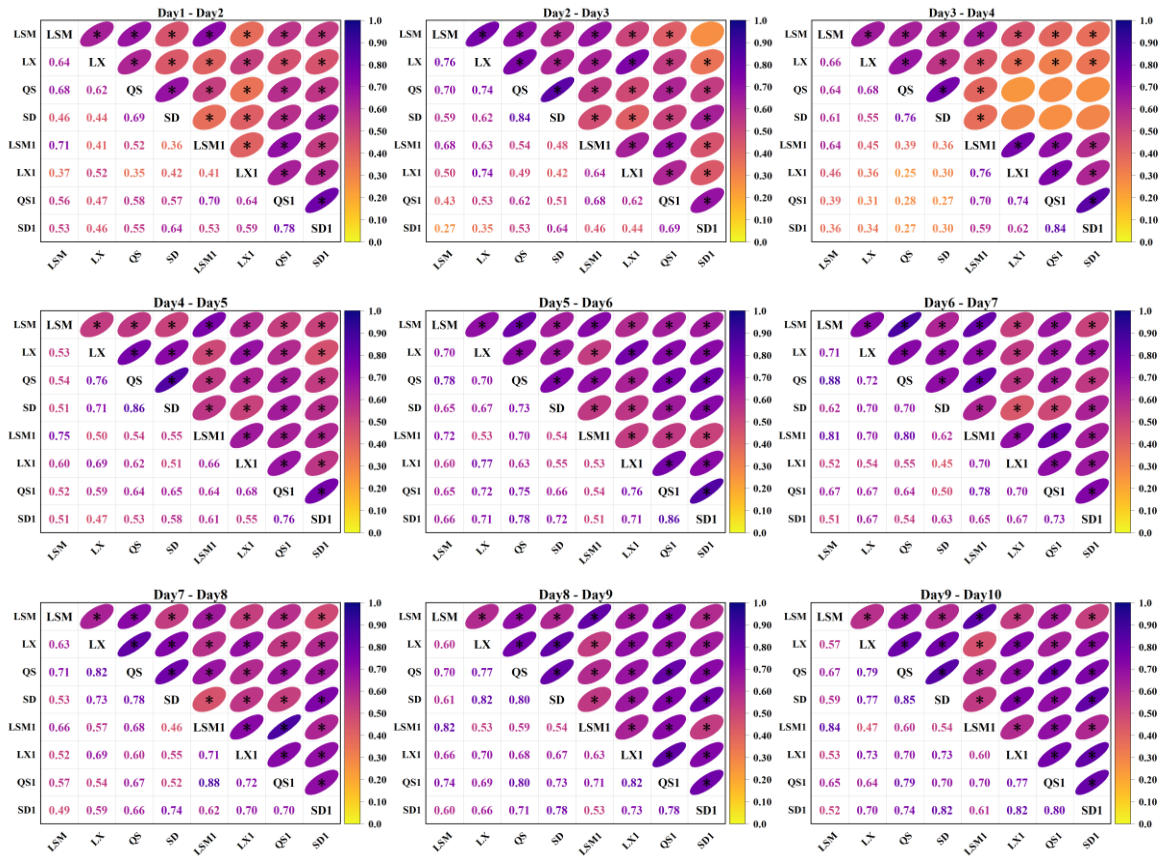
523 Figure 109. Partial results of correlation analysis for daily runoff at multiple sites (LSM, LX, QS, SD 524 represent the runoff sequences of current day, while LSM1, LX1, QS1, SD1 represent the runoff sequences 525 of previous day)
