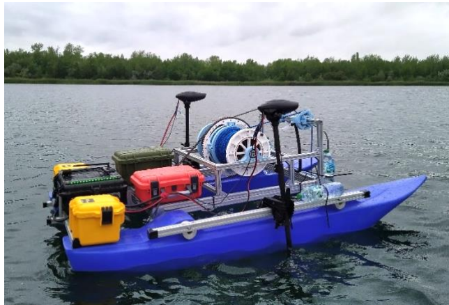
Fig. 1. An expanded implementation of the MARP-FG concept supports a payload capacity of 100 kg. This enables the platform to carry an ultrasound scanning system or, shown here, a winch with a multisensor probe capable of descending to depths of up to 70 m water depth. The thrusters are Minn Kota electric drives
