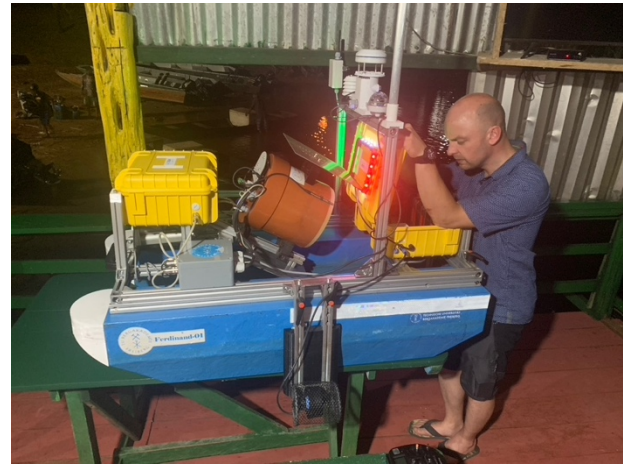
Fig. 2. a) MARP-FG with chamber system. On top, communication antennas, and micrometeorological sensors for wind, humidity temperature and precipitation (white). Below the bridge, at rear, the chamber-tilting mechanism, and the automatic gas sampling box 2 (yellow). Two thrusters are mounted at the center. The chamber (open during transport and flushing) sits in the center inside (orange); deflector shields are visible (gray). In the front: Power supply and positioning equipment in box 1 (yellow). b) The real MARP-FG prior to a launch. See text for more detail
