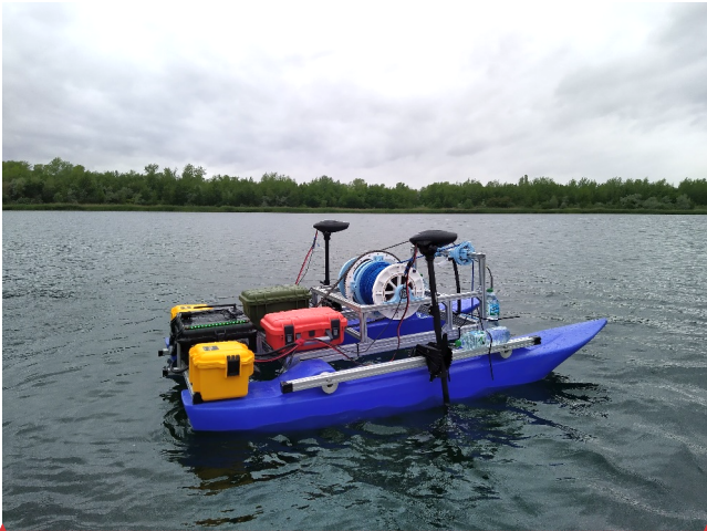
Fig. 1. An expanded implementation of the MARP-FG concept supports a payload capacity of 100 kg. This enables the platform to carry an ultrasound scanning system or, shown here, a winch with a multisensor probe capable of descending to depths of up to 70 m water depth. The thrusters are Minn Kota electric drives
