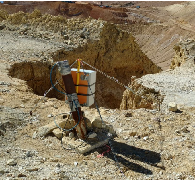
245 Figure 3: Photograph of borehole 5-1 showing erosional gully that formed during the 2015 calendar year.
