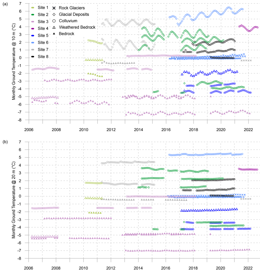
Figure 5: Monthly ground temperatures at depths of 10 m (a) and 20 m (b) at boreholes with at least a full year of measurements. Measurements in bedrock and in rock glaciers are plotted every two months for clarity in the figure.
