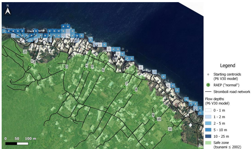
160 Figure 2: Establishment of baseline data: starting centroids for the numerical simulation of a 30 million m 3 tsunamigenic landslide that detached from position number 6 (294 m below sea level) with a density of volcanic materials of 2.5 kg/m 3 , Stromboli road network and Refuge Area Entry Point, to run evacuation models. Map was produced by the authors using Quantum GIS version 3.16.7 software (2021).
