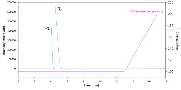
Thermal Conductivity Detector + RT-MSieve 5A Column
