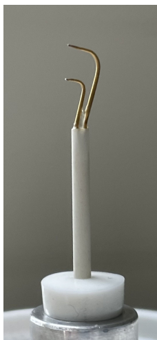
Figure 1. UFT-2B head sensor. A parallel to the mean flow, tungsten wire (2.5 \mu\text{m} thick, 3 mm long) spanned on miniature industry-standard wire probe by DANTEC®.
