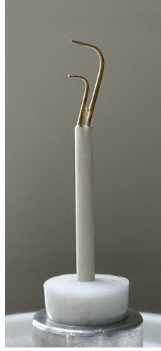
Figure 1. UFT-2B head sensor. A parallel to the mean flow, tungsten wire (2.5 \mu\text{m} thick, 3 mm long) spanned on miniature industry-standard wire probe by DANTEC®.
