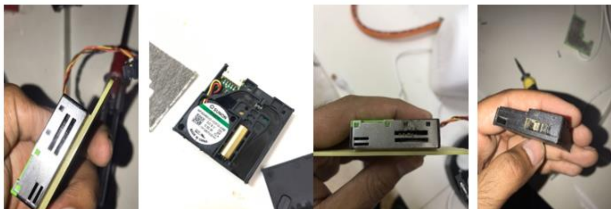
Figure 5: Cleansing mechanism of PM Sensor component of BlueSky 8143 Air Quality Monitor
