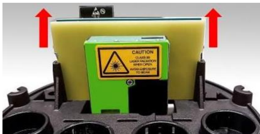
Figure 4: Sensirion PM Component disassembly procedure for cleansing purposes (Image Credit: TSI Bluesky Manual)
