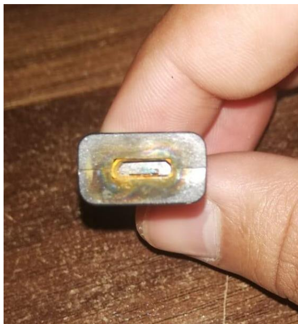
Figure 12: The worn-out rusty female USB B type pin of y splitter attached with Wi-Fi Dongle in Islamabad
