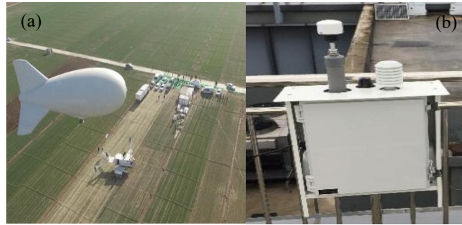
Fig. 13 (a) Field campaign at Wangdu County during December 2018; (b) MAS-AF300 air quality monitoring system.
