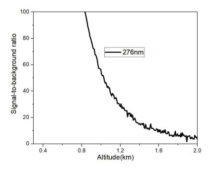
So it is only used in ozone retrieval under 600 m altitude. Above 600m, we adopted the wavelength pairs of 287.2 nm and 299.1 nm for ozone detection.
