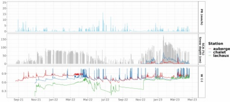
Figure 6. Soil moisture measured at 25 cm depth at the three measurement points, together with precipitation recorded at Auberge station, the MOD10A1 daily values of Snow Cover Area, on average over the entire catchment and the snow depths estimated at the SnowTree instruments at Auberge and Chalet spots.
