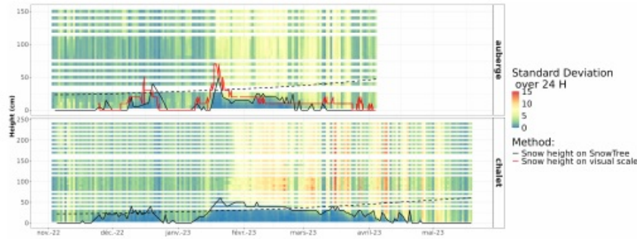
Figure 2. Temperature standard deviation computed over 24 h ( 24hSTD ) recorded by the iButton loggers on the SnowTree instrument at the Auberge and Chalet locations (background colors). Black and red solid lines represent the snow depths obtained from the SnowTrees and the visual scales, respectively. The dashed line corresponds to the intensity of solar illumination received at the measurement points. The solar illumination in the valley, including hill-shading effects is computed with the hillshading function ( insol R package; Corripio and Corripio, 2019).
