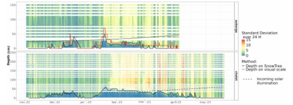
Figure 2. Temperature standard deviation computed over 24 h ( 24hSTD ) recorded by the iButton loggers on the SnowTree instrument at the Auberge and Chalet locations (background colors). Black and red solid lines represent the snow depths obtained from the SnowTrees and the visual scales, respectively. The dashed line corresponds to the intensity of solar illumination received at the measurement points.
