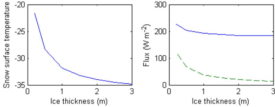
**Figure 4.** Sensitivity of snow surface temperature (left panel), conductive heat flux through snow and ice (right panel, dashed line), and upward longwave radiation (right panel, solid line) to sea-ice thickness and snow depth (set as 10 % of the ice thickness). The numbers are representative for February in the central Arctic Ocean.
