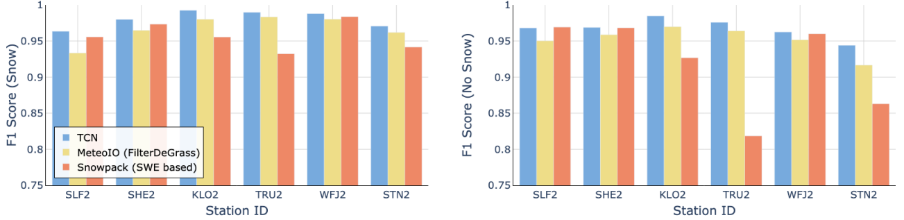
Figure 12. Comparison to other approaches shown as performance (F1-score) per station for CleanSnow (blue), the filter based on the SWE from SNOWPACK (red) and the thresholding filter from MeteioIO (yellow).
