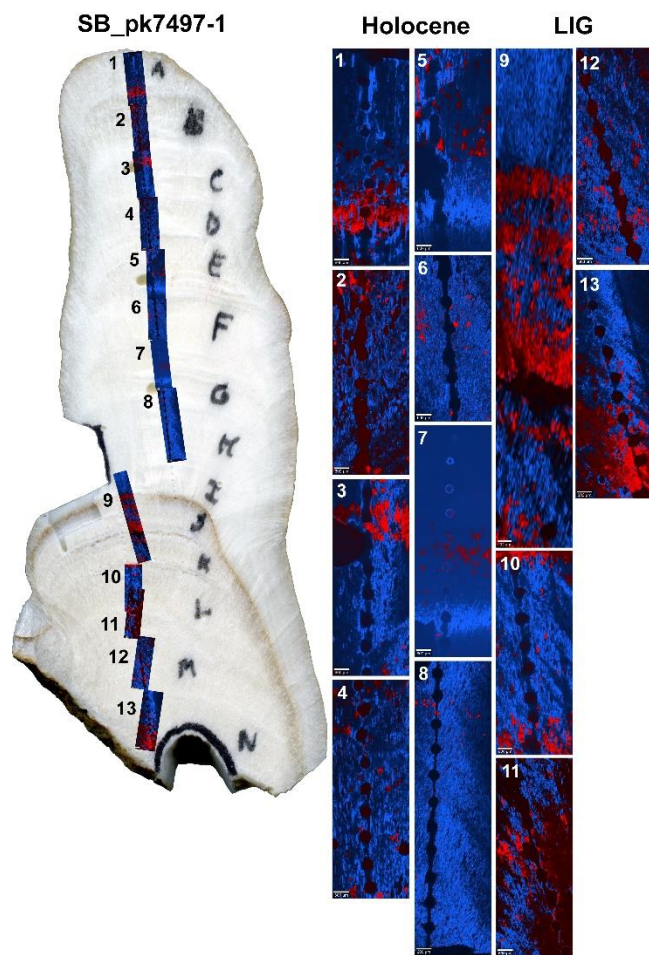
790 Fig. C: All Raman maps and corresponding locations presenting aragonite (blue shades) and calcite (red shades) mineralogy along the growth axis of sample SB_pk7497-1.
