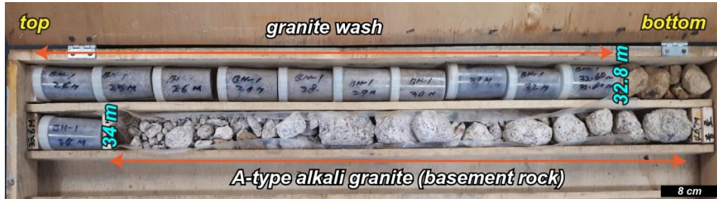
695 Figure D1: Photograph showing drilled core. The lowermost of the unconsolidated sediments, the granite wash, directly overlies bedrock. Cosmogenic ^{10}\text{Be} - ^{26}\text{Al} isochron dating samples are taken from this granite wash.
